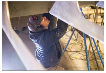
Leigh O'Conner works on the extension of the Kariel's stern, which will help to increase floatation to improve the boat's safety and efficiency.
